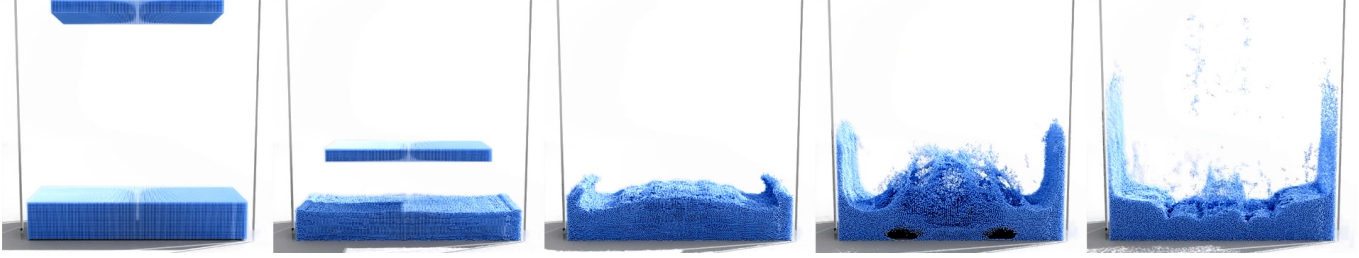
Fig. 11. The Block Flop example with 250K particles simulated using our IPBF method. A block of fluid drops onto a puddle. The resulting simulation results in a period of high density error, but with 2 iterations and a time step size of h = 1/240 , we maintain stability with incompressibility, running at an average of 60 ms per frame.
