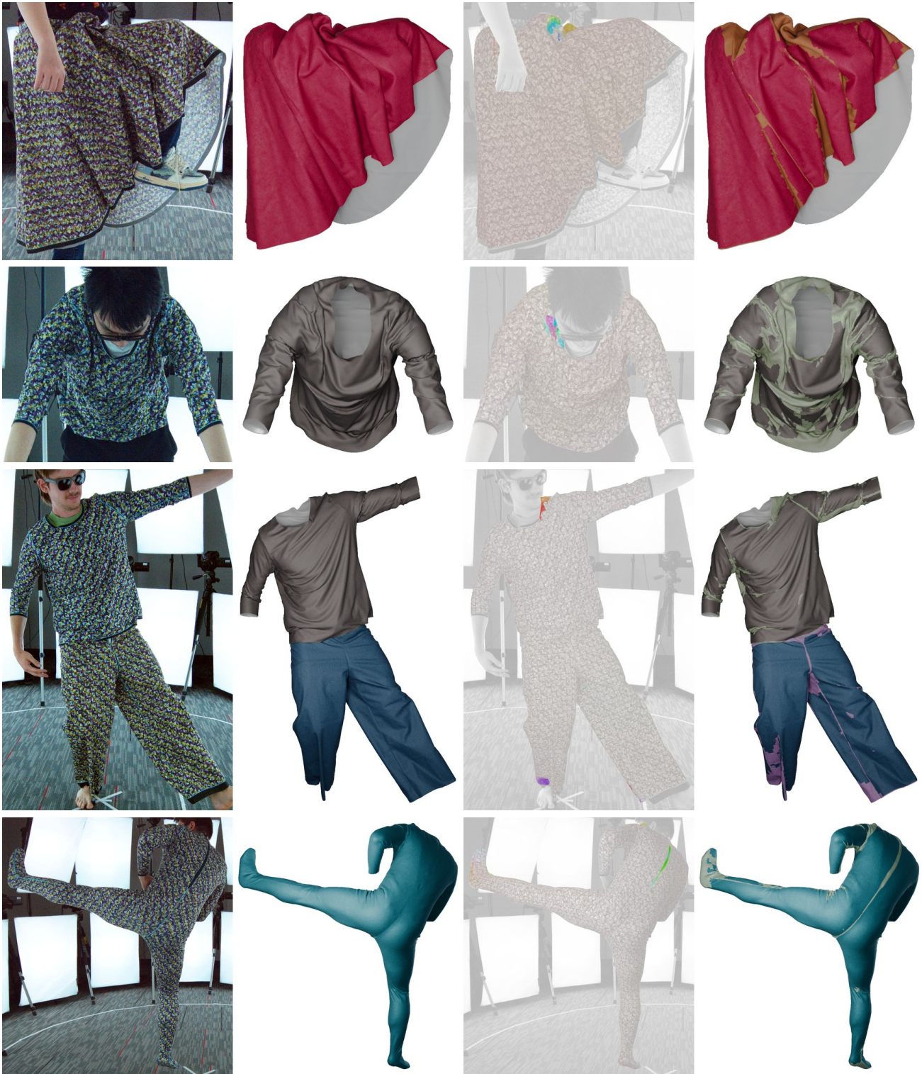
Fig. 9. Challenging examples from all four capture sequences. In addition to the input image and full reconstruction (left two columns), we show the optical flow between the input image and retextured reconstruction (third column) and the highlighted inpainted regions (fourth column) for comparison. Color hue denotes optical flow angle, while intensity denotes magnitude.
