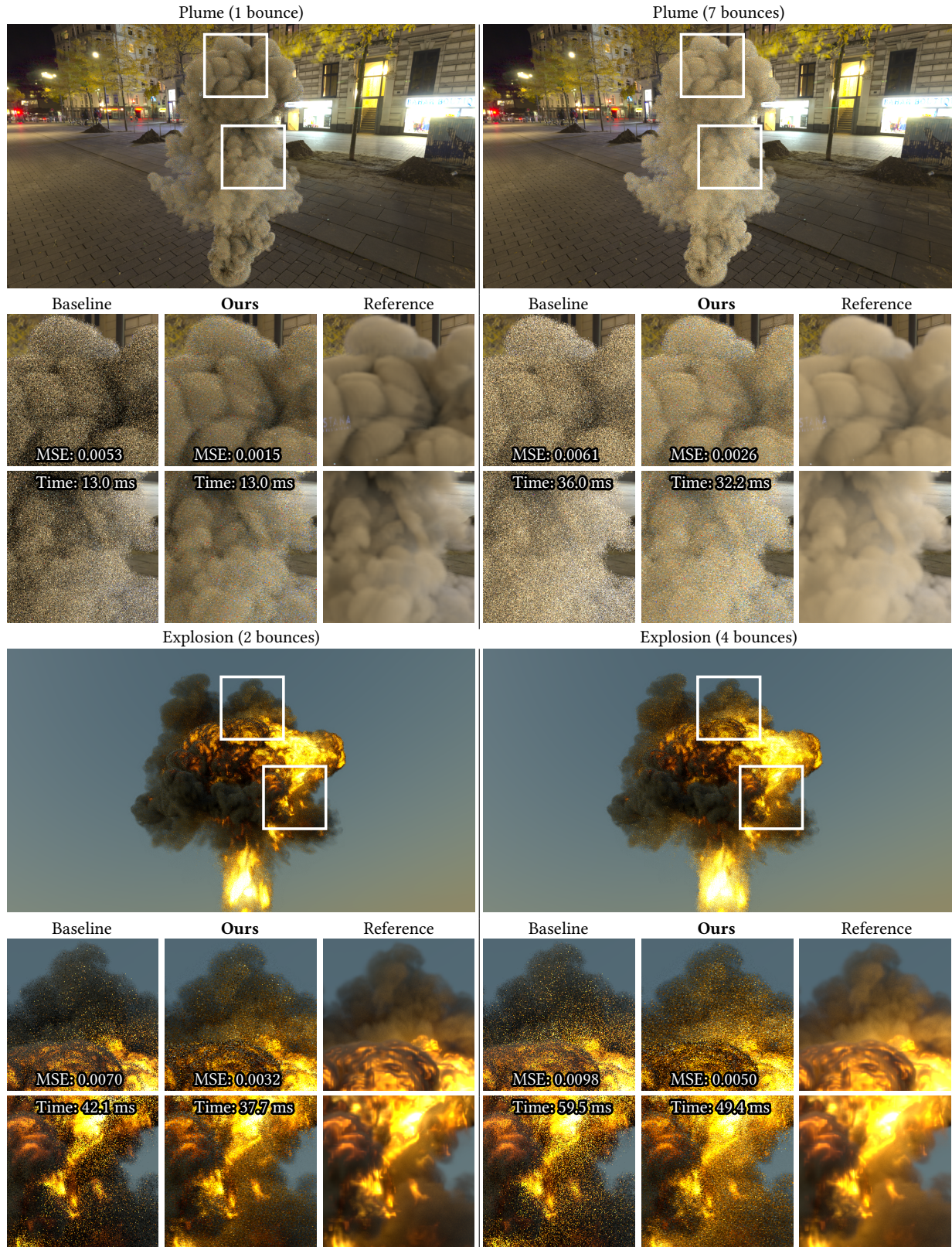
Fig. 17. The Plume and Explosion scenes, with roughly equal-time comparisons between the baseline and our method.
